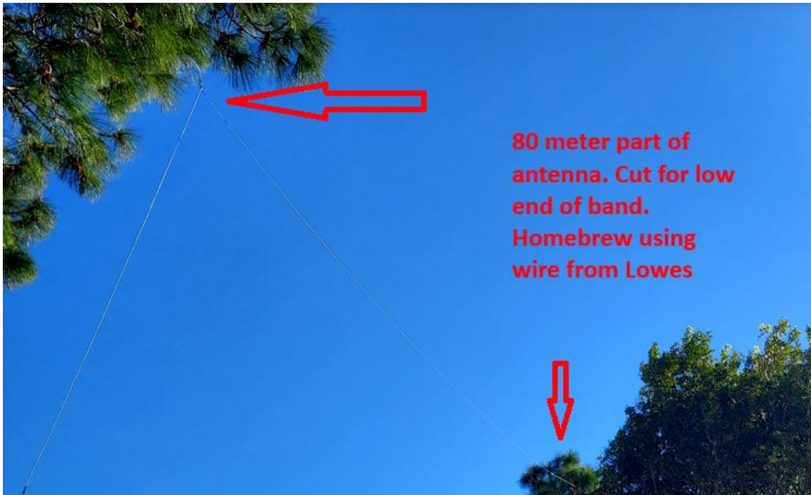
Inverted L antenna - Giving low angle of radiation. Outstanding DX on 160-80-30-40-15-10 m
