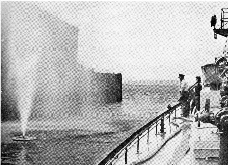
PUTTING DOCK FIRES ON THE SPOT —New device for fighting fires under piers, directs a powerful stream of water upwards. It is controlled from the fireboat
