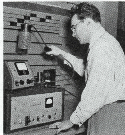
Engineer P. Bencivenga sets up a Geiger-Muller counter to measure intensity of ionization during a recent research project
