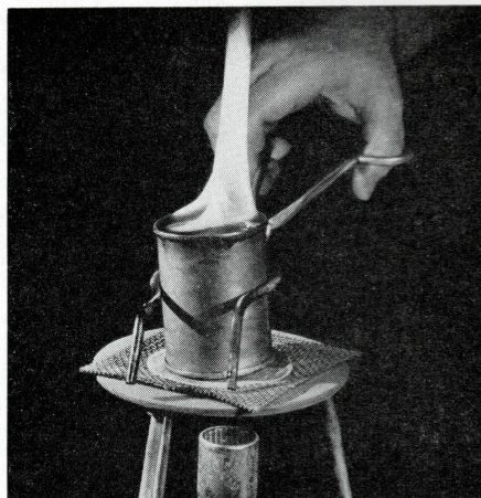
VAPORS IGNITE — Paraffin wax is heated until it is hot enough for the vapors to ignite. The heat is then removed, as shown in the illustration at the right, to show how fires of some types can be extinguished by the process of cooling the burning substance
