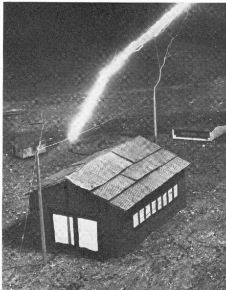
LIGHTNING "UMBRELLA" — Man-made lightning, streaking toward a model high explosives plant at the Westinghouse Laboratory in Trafford, Pa., is deflected by a wire "umbrella" which guides it harmlessly into the earth
