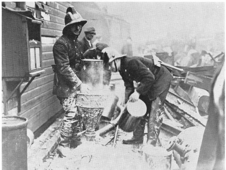
MODERN METHODS —A new type of foam is mixed with water from the hose to subdue stubborn chemical fire at a recent blaze in a tar distillery at London, England
